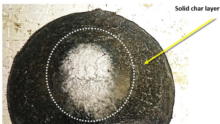
Figure 10. CN 10 sample after ablation test
