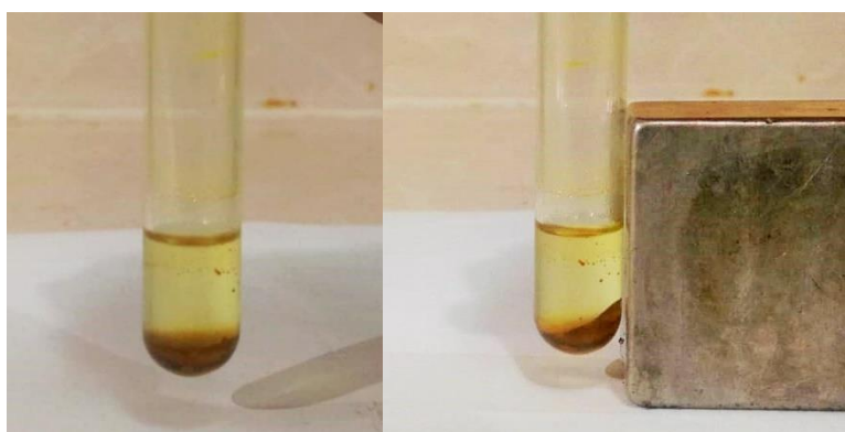
Figure 9. [\text{C}_4\text{py}]\text{FeCl}_4 deposited at the bottom of a glass tube and attracted to a NbFeB magnet
