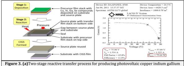
selenide (CIGS) film. Cu: Copper. In: Indium. Ga: Gallium. Se: Selenium. **(b)** Light current-voltage (IV) curve measured by the National Renewable Energy Laboratory (NREL) on a 120×60cm<sup>2</sup> CIGS module.
