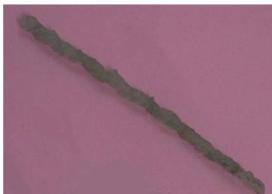
Figure 3. The polypropylene extrusion with copper pigment.
