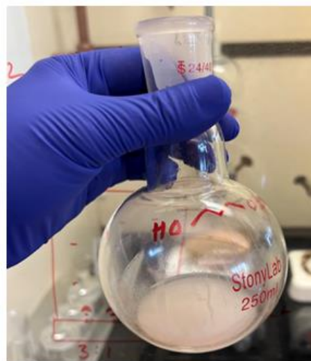
Figure 3. Precipitation method used in purification step.
