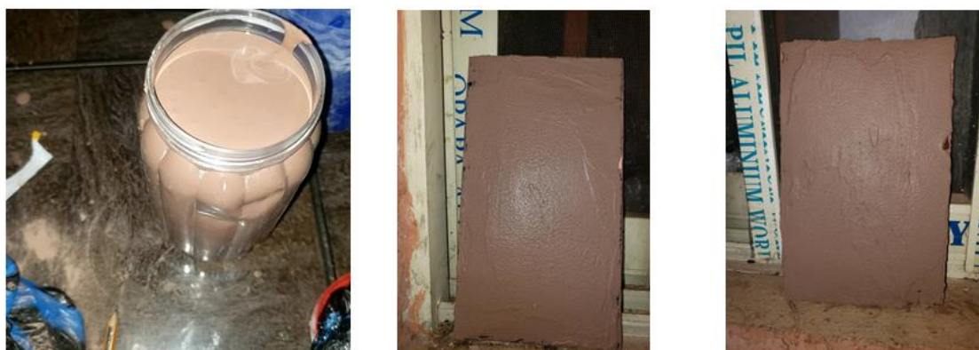
Figure 2. (a) Produced screeding paint, (b) screeding paint at 450 °C, (c) screeding paint at 750 °C.
