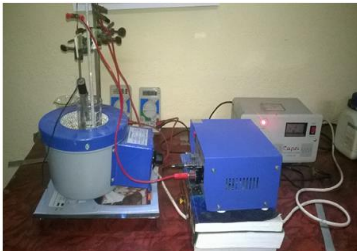
Figure 1 (b). Galvanostatic linear electrodeposition setup.
