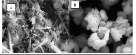
**Figure 6.** Representative TEM image of (a) the assynthesized CuMOFs (b) CuO embedded in carbon matrix
